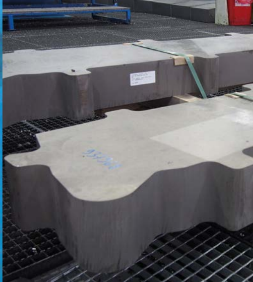
Rough stock spars ready for machining by the ASPX
