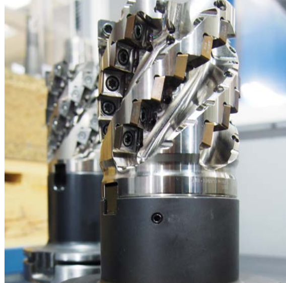
ASPX milling cutter in the foreground; VFX milling cutter in the background.
