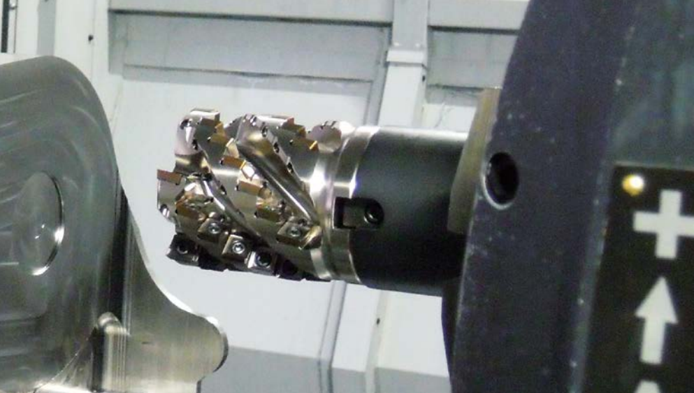
ASPX milling cutter ready for machining
