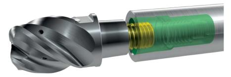
3 The iMX end mill from Mitsubishi Materials, the shank and cutting head are both made of carbide. The stable taper and clamping surfaces give the tools a strength which comes close to that of solid carbide mills [photo: MMC Hartmetall]
