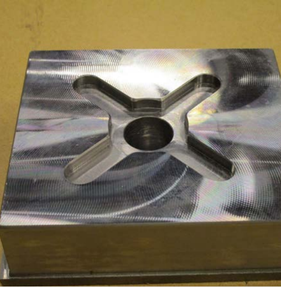
Part machined female modular clamping component
