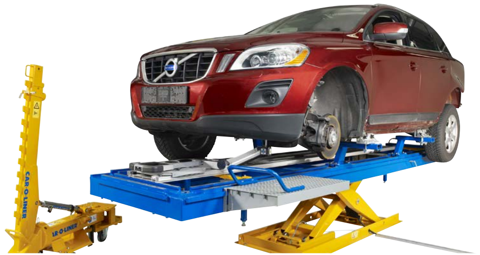
The Car-O-Liner bench in use - Establishing the extent of the mis-alignment damage
