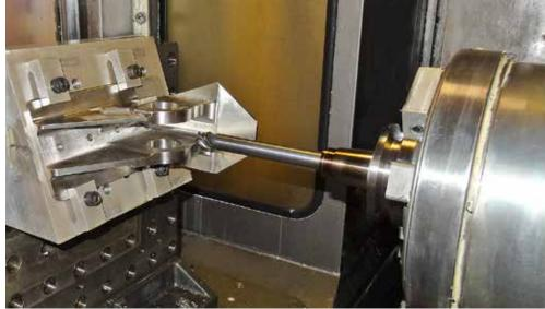
Brace machined by Mitsubishi Materials iMX exchangeable head end mills
