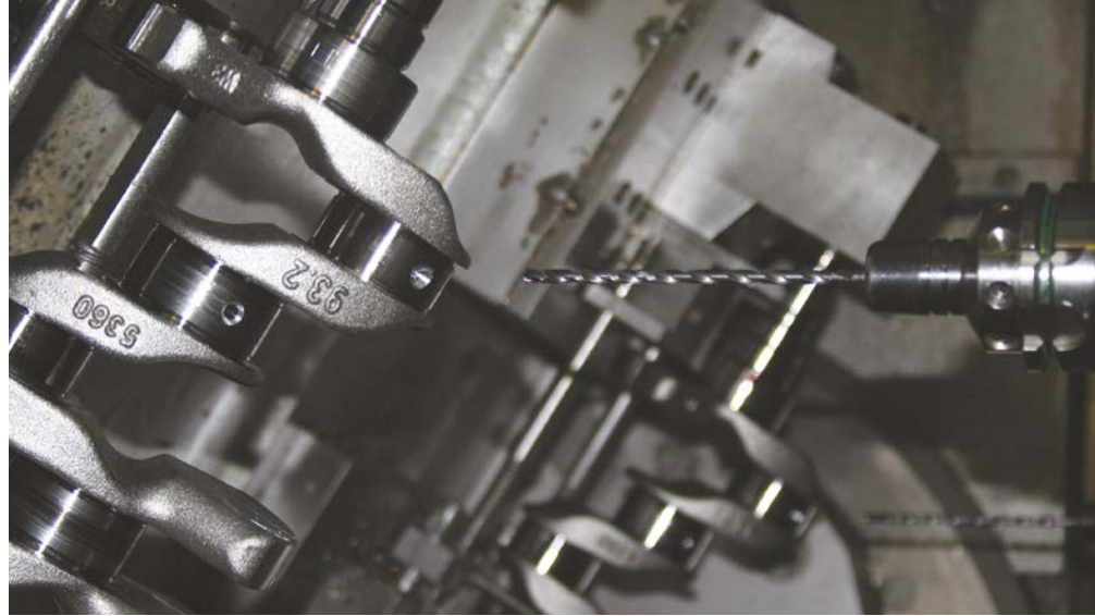
MPS1 - Pin journal through to main bearing journal deep hole drilling on a twin spindle Grob BZ530 machine
