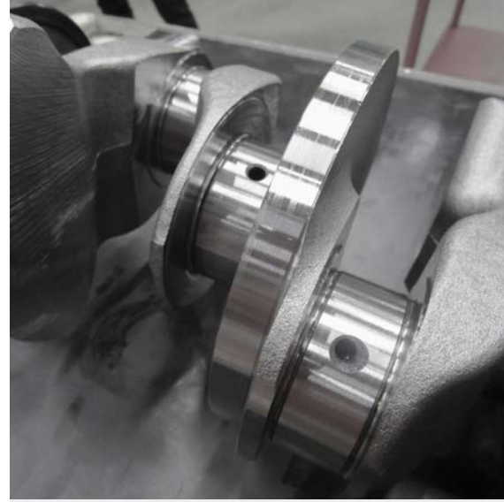
Diagonal hole Ø5.00 mm, 100 mm deep.
