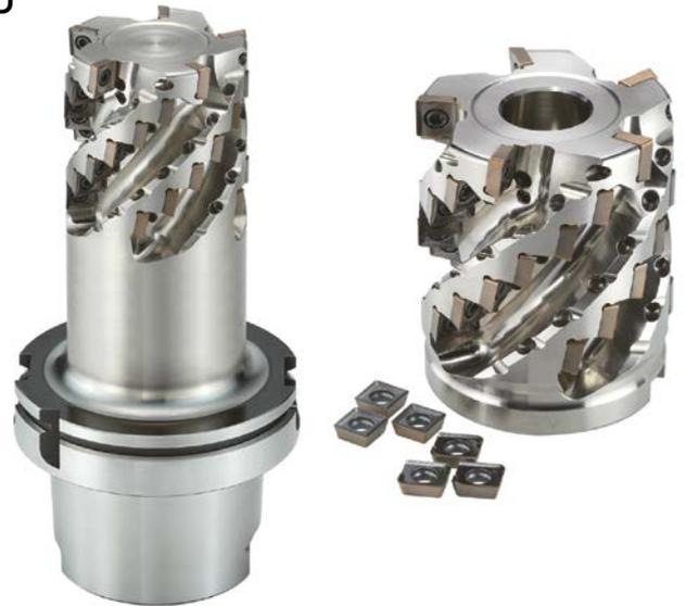
ensure a smooth but strong cutting action. In combination with a JM edge honing that enhances the low cutting resistance, the inserts provide all the features necessary for reliable, high performance machining.
